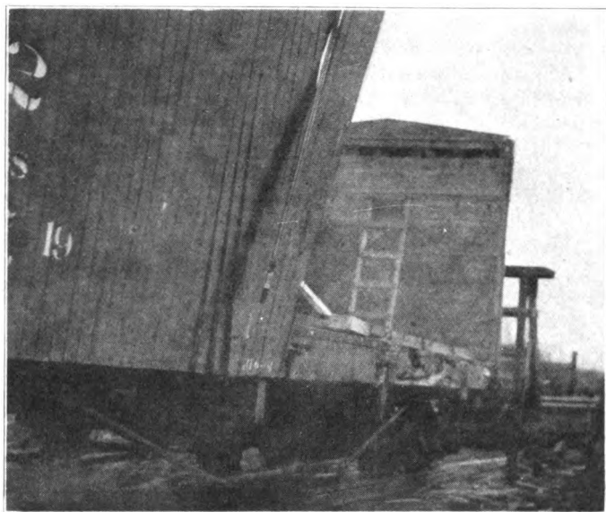
Fig. 4. Furniture Car as Received for Repairs.
